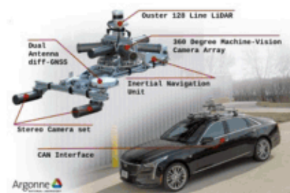
APACK-V high-resolution multi-sensor on-road DAQ
