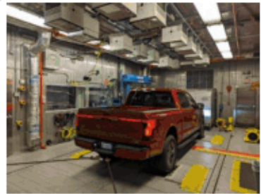
4WD Light Duty Chassis Dynamometer & Thermal Chamber
