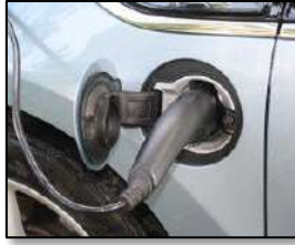
SAE J1772 Standard Level 1 & 2 Charging Connection (Left) and Plug (Right) US EVs
